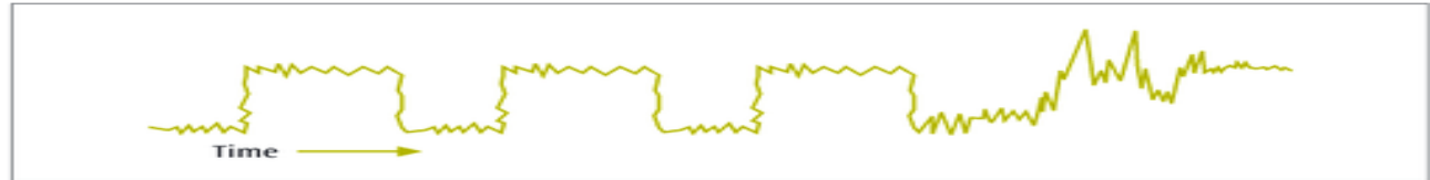
Figure 6-2 The effect of impulse noise on a digital signal
